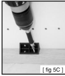
Attach corner blocks to both side of the cabinet, see figure 5D
