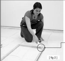
Place face frame "A" face down on a smooth surface to prevent scratching (you may use the box it came in). Glue all female dovetail joints as shown in fig. 2. Slide shelves "D" into position while aligning as in fig. 2A & 2B with holes closest to the face frame.
